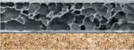
BikeShare Helmet Cross Section
